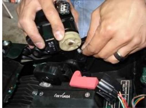
4. Pull the cable through from below, replace the servo motor, reconnect the wiring, and clip the connector back in to place.
