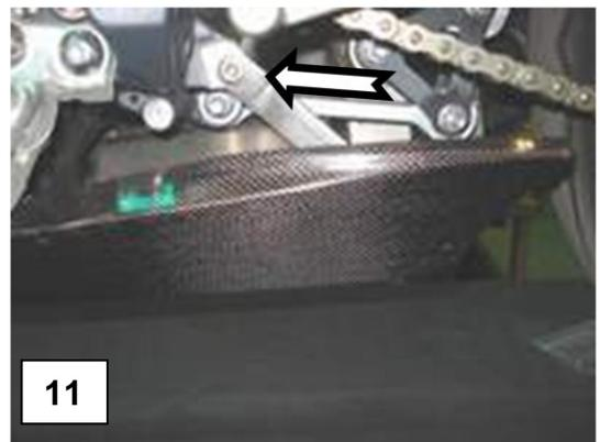
13. Align the hole in the rear of the trim with the hole in the trim bracket (you can use a small awl or screw driver to help line up the holes).
