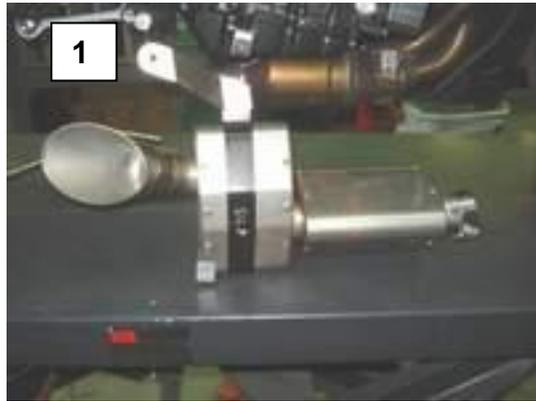
2. Slide the muffler onto the stock headers as far as it will go. A little light oil inside the muffler slip joint will help to ease the muffler onto the header. The strap mounting bracket is positioned behind the stock mount of the rider's footrest plate.
