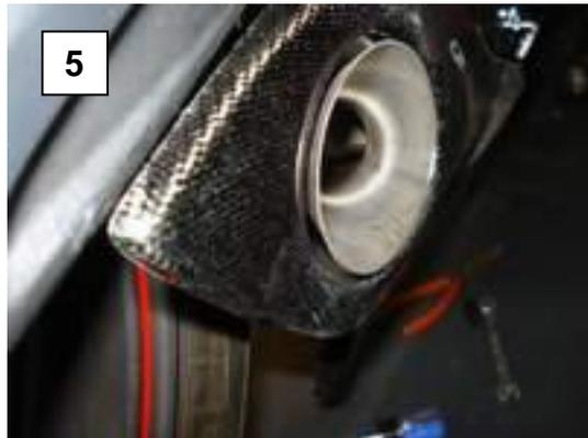
Now check the alignment of the exit with the trim. Make any adjustments necessary following the alignment guide at the start of this section. It may be necessary to remove and refit the trim more than once to achieve the perfect fit.
