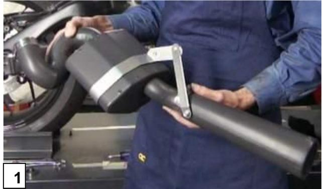
3. Return rider's footrest into position and tighten mounting bolts finger tight.
