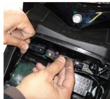
3. Remove the bolt securing the servo motor to the under tray. Pull the motor off its post and disconnect the cable.
